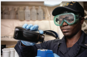
FIGURE 4: This mechanic tests the viscosity of an oil sample. If the viscosity of the oil is too high or too low, it could cause damage to the engine.
