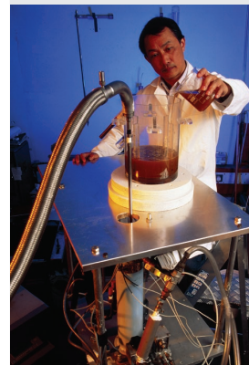
FIGURE 18: In this device, bacteria are used to remove nuclear waste ions from a biological sample.
